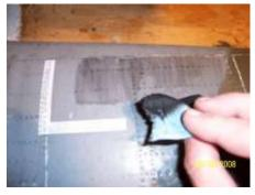
I then wipe this mixture on the entire aircraft. Front to back on the wings and stab, and top to bottom on the fuse and vertical fin. I don't do the entire plane at once, I will work in sections at a time. When wiping the black mixture on the plane, I will make sure I get it into all the rivet detail, hatches, panel lines etc that I want to highlight. After about a minute or less, you can then wipe the mixture off.
