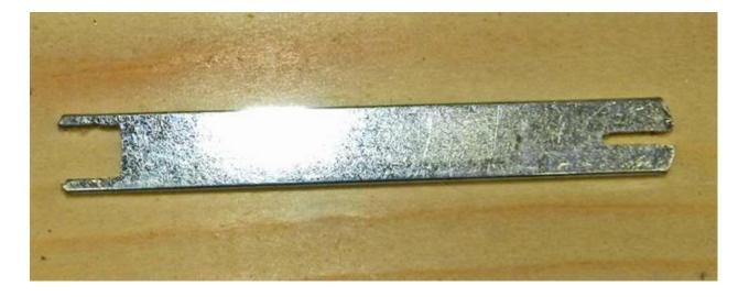
One end turns the flat steel rigging and the other end turns the lock nut. All very simple to make.
