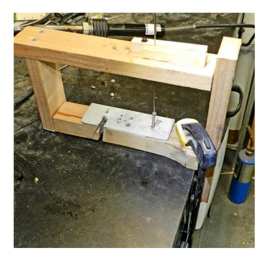
The screw is inserted into the hole in the alloy part and the rigging is slid into a slot in the top part like this.
