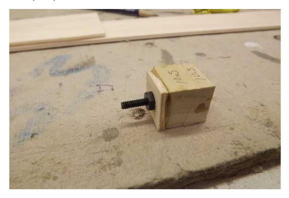
After the glue has set, drop the 1-1/4" bolt through the brass tubing and out of the washer on the end. Insert the bolt though one half of the block, the two ribs, and into the block with the blind nut. Snug it up to the ribs and apply liberal thin CA to the two blocks. Apply non-sag 5-minute Hysol to the brass tubing and washer to bind them to the rib.
