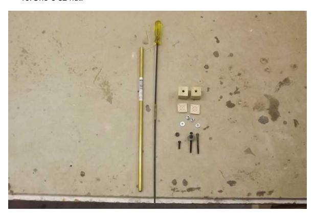
Make a jig to hold the brass tubing perpendicular to the washer. Use the short 6-32 bolt to center the washer over the hole drilled in the base of the jig.
