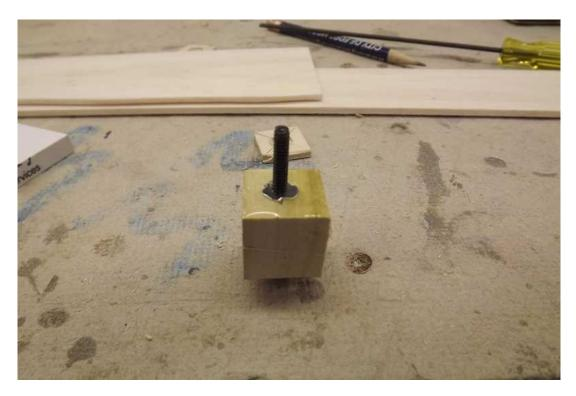
Place the capture plate over the blind nut and secure with the 6-32 nut.
