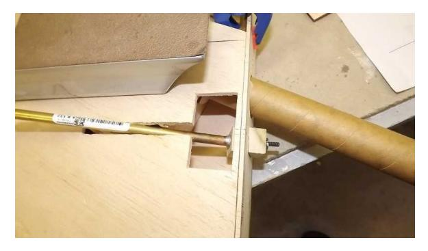
Add 1/4" square balsa sticks to the sides of the brass tubing for support. Keep them flush to the top of the ribs.
