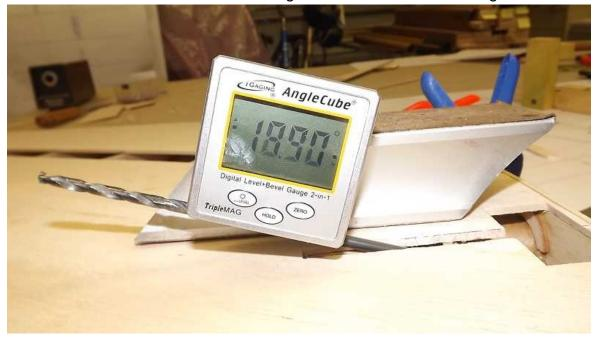
Mark the center line of the block, Shim the angle cube to the correct angle and draw a line on the block equal distance from the top and bottom center lines.
