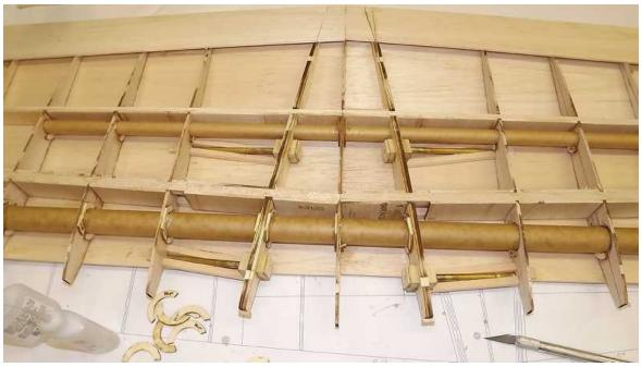
After sheeting around the tubes, cut them off flush with the surface using a Dremel cutting wheel. Fill around the tube with wood putty.
