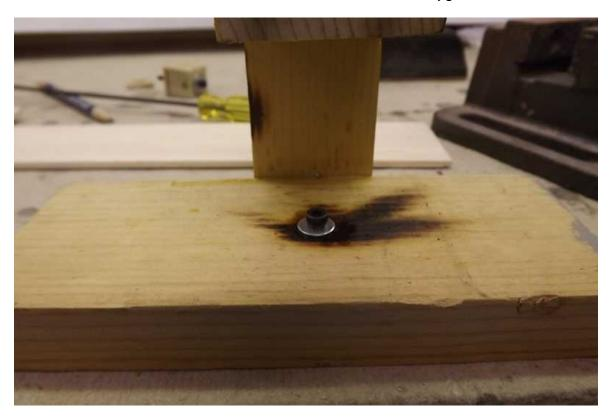
Solder the brass tubing to the 6-32 flat washer.
