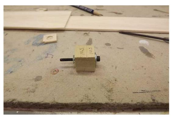
Put 5 min epoxy under the blind nut and around the block surface. Tighten the bolt to secure the blind nut.
