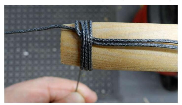
In this example this is as far as the binding is going, on yours it should be long enough to cover the length of the metal insert.
