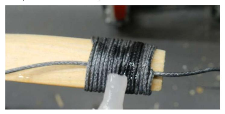
Carefully cut of both ends of the thread with a sharp Xacto knife and it should look like this No Knots, no loose ends!
