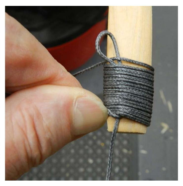
Now put a small drop of C/A on that place where the line and the loop are and if the strut tapers at the bottom another drop there to secure it.
