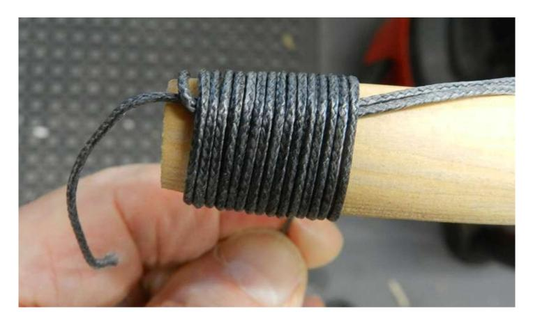
Now thread the binding line through the loop.
