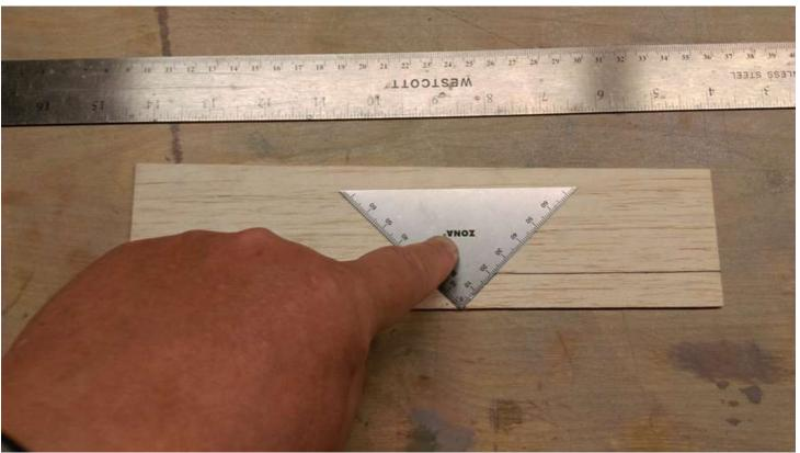
Again it's VERY important to stress you HAVE TO HAVE THE GRAIN CROSSING THE JOINT at 45 degrees. Here is the gussets all drawn out and ready to cut out.
