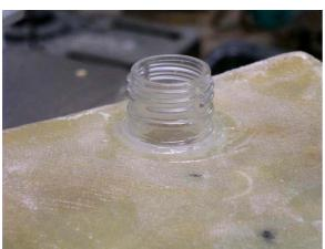
I used the top of a 1.5 liters Soda bottle so I can attach the tube from the engine, the filler tube and the breathing tube. It was glued into place with the help of Hysol, 5 minutes.
