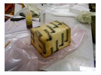
6 layers of 163 gr/sq meter glass cloth and Pacer Finishing resin later....
