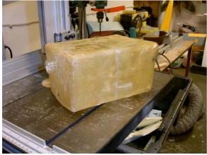
When the Hysol was cured, Iglued the two halfes together with some more Hysol. Then I wraped the seam with a couple of layers with 163 gr/sq meter glasscloth and some more Finishing Resin.
