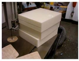
Then I cut enough foam to make a block slightly bigger than the dimension I have available. I glued these blocks together with some waterbased contact cement. When it had cured, I drew a centerline around the whole block and nailed the templates to the shortends of the foam block. When this was done, it was time to remove all the excess foam with the help of a hot wire. This could also be done by sanding. It will just take a little longer
