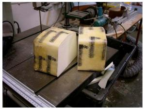
When the epoxy was cured, I cut the plug into two pieces.
