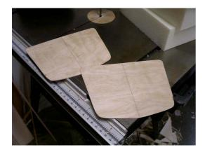
The first thing I did was measure how large the space is and out of this I made a simple sketch. Now I knew the dimension I could use so I made two templates out of plywood. These templetes was used to get the right shape on the plug.
