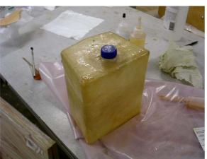
All that had to be added now was the cap from the soda bottle. The fittings so you can attach the tubes to the tank was made out of a small kit from the local hobby shop. It contained all the things I needed to make the attachments.
