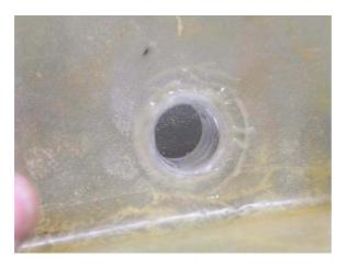
The inside of the bottle top was sealed with some more Hysol to make sure there would be no leaks.
