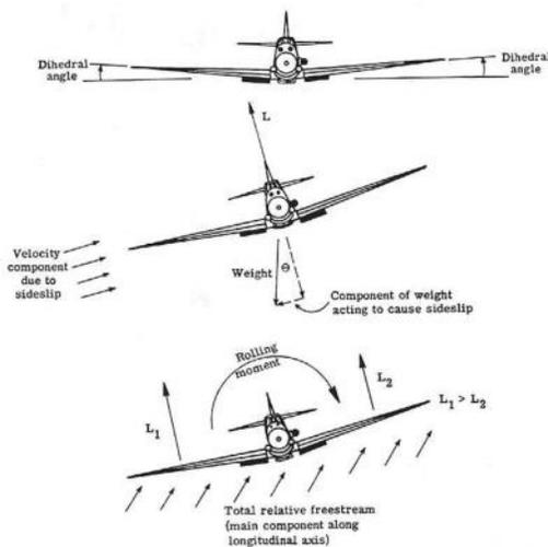
When an aircraft is disturbed from an upright position, it will sideslip toward the down-going wing, increasing airflow along the length of the wing from tip to root. The dihedral angle increases angle of attack to this lateral flow, generating additional lift to restore the aircraft to a level attitude.
