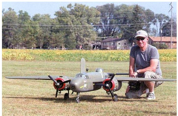
Richard Steine's B-25 has no dihedral in its outer wing panels. Unwanted yaw and roll are minimized if one engine fails. Mid-wing configuration plus inboard dihedral raises the center of lift above the center of gravity, producing pendulum stability - a brilliant balance of compromises. Appearance of negative dihedral is an optical illusion.
