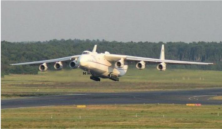
Anhedral in the Antonov 225 compensates for its extremely low center of gravity and reduces unwanted yaw and roll in the event of engine failure.
