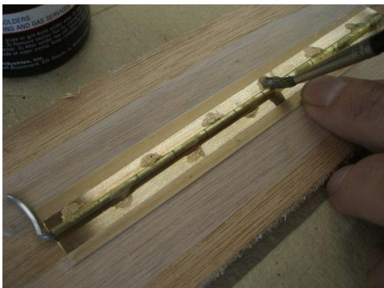
Hinge pin with tubes.
