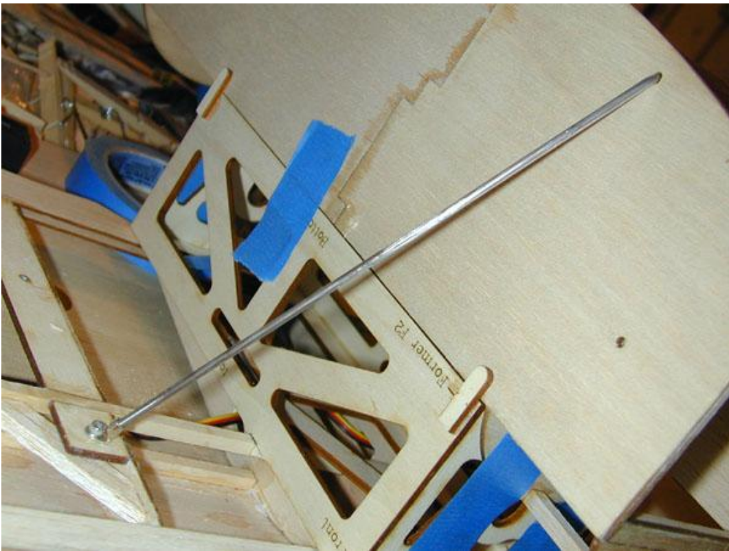
With the wing and fuselage turn up-side down, The struts are cut to length, bent to shape and positioned with the solder lug screwed to the wing.
