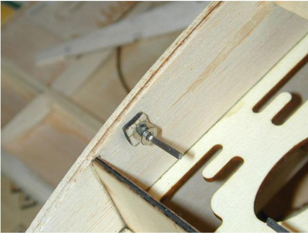
To make the cabane struts removable, I used lock collars to secure the wires in the fuselage.
