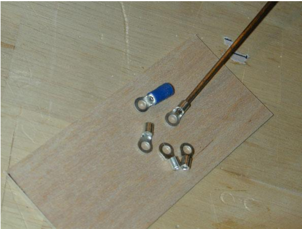
An old school technique is to use solder lugs at the top of the music wire struts.
