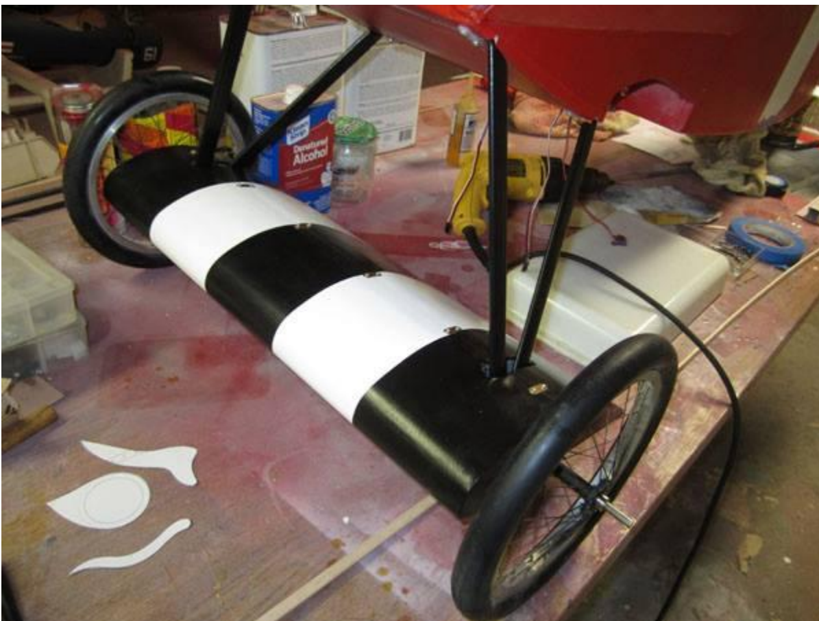
Nothing fancy here, now just sand and fill and prime and repeat. When all the pin holes are filled, finish sanding with 320 grit and repaint your sub-wing. Allow to dry then go out and do some more flying!
