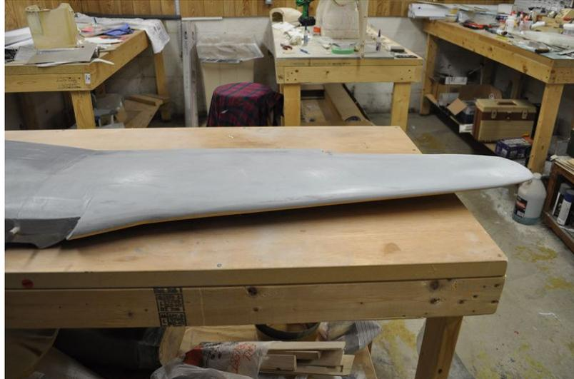
Above this is the wing with the first coat of primer applied.
