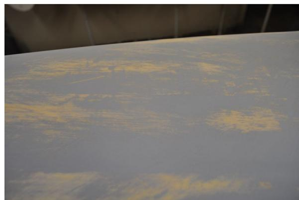
After a good first sanding this is about what you will end up. It is hard to tell in the pictures above but you will end up seeing some of the fiberglass weave. The spots that look like bare wood are not sanded through the fiber glass. Be careful not to sand through your fiberglass cloth.
