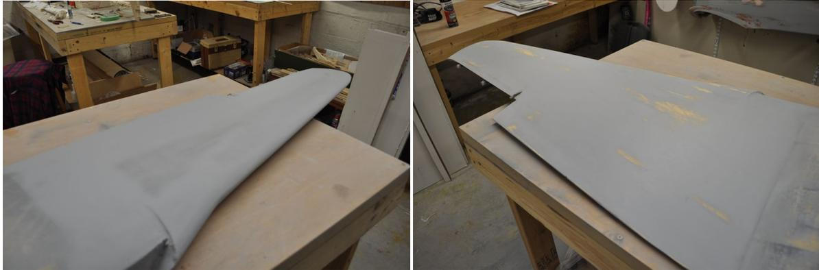
As before and after, the same process of sanding is used. Depending on the how you applied the fiberglass and other conditions more coats or even less coats may be required to fully fill the weave.
