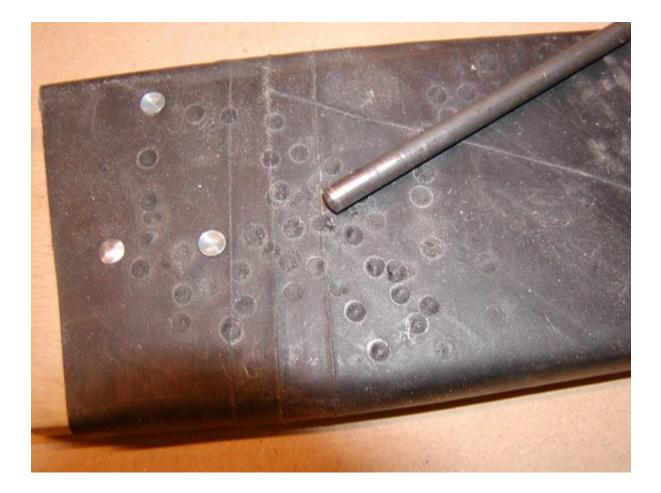
If you want shiny unpainted rivets, polish a handy size piece of litho -thin or medium, thick before you start. If you rivets will be painted, stamp the printed side down. Bring the punch down in a snap. With a little practice you can here them snap out.
