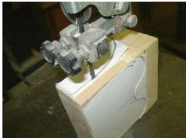
Cut the side view with a bandsaw.
