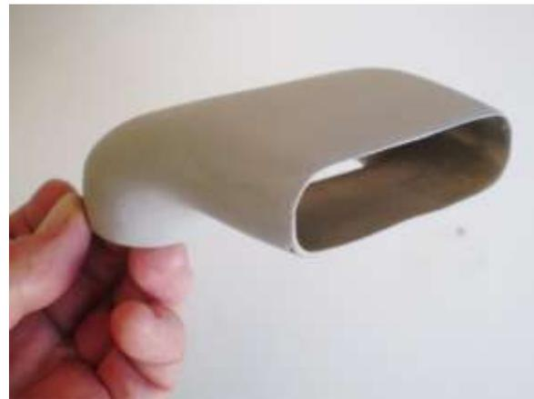
Sand the surface. Drill out the balsa core. Continue removing the core with an X-Acto knife, file, sandpaper etc, leaving nothing but the fiberglass covering. This is known as the “lost wax” method.
