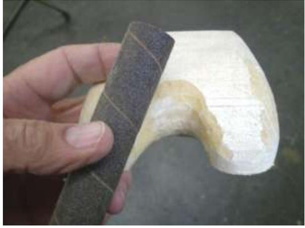
Round the edges using an X-Acto knife, sanding spindle tube, sanding block and sandpaper,
