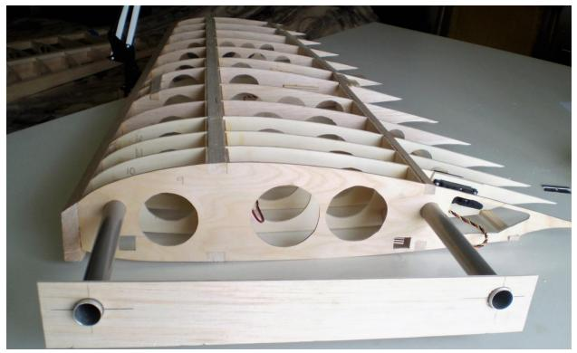
A giant scale airplane can have as many as two dozen rib sizes. It is possible to draw each of these ribs manually but that method is not very accurate. The process needs to be precise for the wing sheeting to mate well with the ribs. A quicker and more accurate method is to use CAD (Computer Aided Design) to draw at least the outline of each rib and the modeler manually draws the remaining details such as spar notches, lightening holes, servo mounts, etc..
