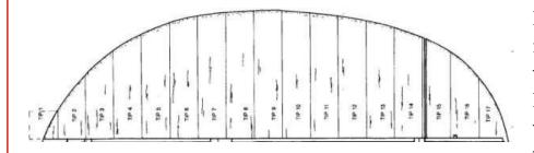
Divide the top view of the wingtip into 1" increments. Measure the wingtip span at each increment. From a drawing of the outermost wing rib, measure the thickness of the wingtip at each increment.
