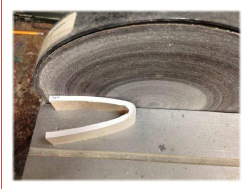
Cut each section slightly outside the line and trim to the line with a disk sander.
