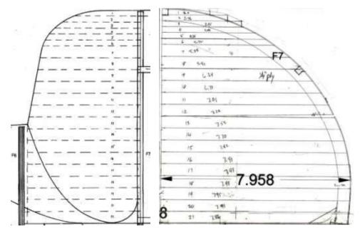
On the side and front views of the windscreen, draw layers 1" and ½" thick, thinner layers where the curve is sharp. Measure and record the length and width of each layer. Because a windscreen is symmetric, you need only measure one side of the top view.
