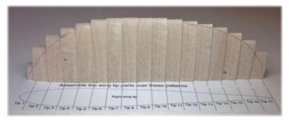
Perform the calculus "limit to infinity" function by planning and sanding away the stepped edge into a smooth shape. Final sanding is accomplished after attaching the tip to the wing.
