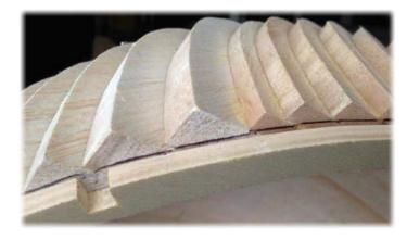
Place the result against the cabin former where the windscreen will be attached and trace the formers outline onto the plug. This will assure an exact fit of the molded plastic windscreen to the former. Trim away the stepped edges, sand to final shape, add fiberglass cloth and primer and wetsand to a super-smooth finish with 1500 grit sandpaper, ready for vacuum forming a clear plastic windscreen.
