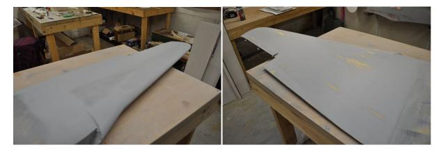
A before and after, the same process of sanding is used. Depending on the how you applied the fiberglass and other conditions more coats or even less coats may be required to fully fill the weave.
