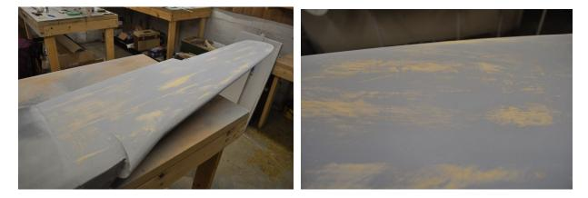
After a good first sanding this is about what you will end up. It is hard to tell in the pictures above but you will end up seeing some of the fiberglass weave. The spots that look like bare wood are not sanded through the fiber glass. Be careful not to sand through your fiberglass cloth.
