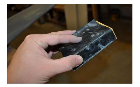
The finer grit sand paper tend to get clogged a little easier, so I am wet sanding this final coat as well. This will help the paper cut as well. It can be a bit messy but you will like the results. You will end up with a very smooth surface.
