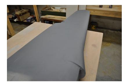
So a fresh coat of primer has been applied. If you notice it has a slightly darker look to it. Just a difference in brands. So for sanding this coat of primer I am going to use a finer grit sand paper. I have 400 grit laying around but 320 works good as well. I probably wouldn't go much below that though since this is the surface you will be applying your paint to. As with above I am using the same sanding sponge and wrapping it in the 400 grit sand paper.
